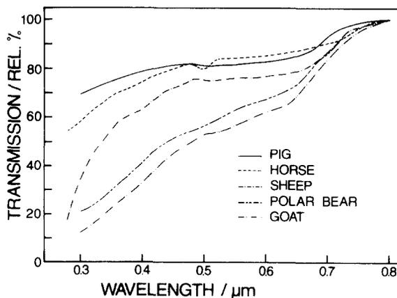
Fig. 3. Comparison of transmission of white hair bundles of different mammals (pig, horse, sheep, polar bear and goat). The value measured at  $0.8 \mu\text{m}$  was calibrated to 100%.
