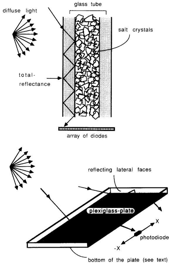
Fig. 1. Set-ups for model experiments on light collection using (top) a capillary with salt crystals forming scattering centers and (bottom) transparent plexiglass plates the bottom of which is modified by defined concentrations of scratches.
