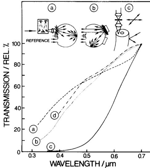
Fig. 4. Transmission-wavelength dependence for hair of polar bear (inserts explain set-ups for measurement): (a) in transmission-scattering, (b) in reflection, (c) transmission of a single hair measured parallel to the hair axis (transmission at 700 nm calibrated to 100%), (d) measurement of transmission of hairs of published by Grojean et al. [2].
