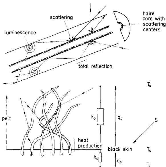
Fig. 7. Scheme explaining scattered light – luminescent light collection in hairs of polar bear and function of pelt as transparent insulation (quantities inserted are described in the text).
