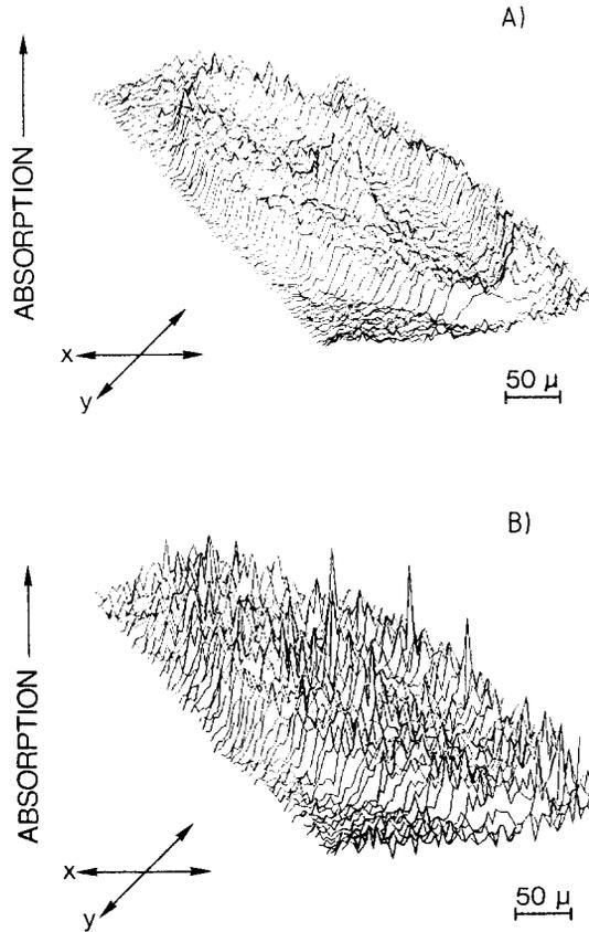
Fig. 5. Scanning light microscope profile of brightness of basal plain of hair of polar bear, computer-processed to an absorption profile: (A) using a W halogene lamp for illumination of a 3 to 4 cm long section of hair; (B) using a xenon lamp.
